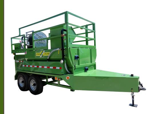
**Bowie's Victor 800** is one of our most popular Hydro-Mulchers. The low maintenance, ease of use and high productivity of the **Bowie Victor 800** Hydro-Mulcher® makes it a smart choice. With its many options, this piece of equipment makes it just right for your hydro-mulching needs. The trailer unit features a tandem 8000 lb. torflex axle, electric brakes on both axles, DOT approved LED running lights and an adjustable ball or pintle hitch.
